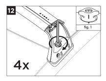
Tighten the wingnuts with the hex wrench (2) until the tower is firmly affixed to the vehicle. We recommend tightening to 2.5-3.5 Nm. To confirm the tower is properly installed, pull in all directions and ensure there's no movement. In order to lock the system, the mark on the wingnut must align with the mark on the tower (see fig. 1).
