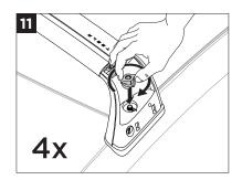
Install the wingnut (11) and hand tighten onto each of the towers.
