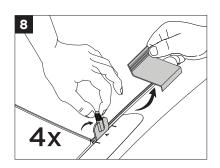
Remove the clip tool (1), being sure the clip (12) is engaged in the metal receiver under the glass. Pull up and wiggle to be sure it's properly engaged. Be sure the center of hook aligns with the arrow
