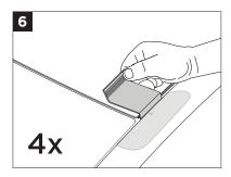
Use the clip tool (1) to carefully retract the rubber gasket at the arrow location.
