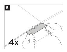
Apply (13) anti-abrasion tape to the front driver side of the vehicle by aligning the arrow on the glass with the arrow on the anti-abrasion tape (13), and aligning the edge of the tape with the edge of the trim line.
