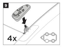
Place the front driver side pad (6) over the clip on the front driver side. Use the icon to help identify and install the correct pad (6-9) in the proper location.
