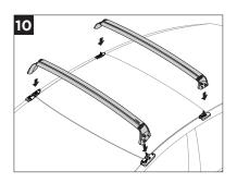
CROSSBAR INSTALLATION: Ensure all four hooks are engaged, properly aligned (step 5-6), and in the upright position. Then, carefully place the front and rear crossbars (4-5) over the pads.
