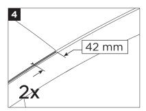
To locate the rear arrows measure 42 mm from the rear edge of the glass top.
