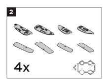
Use the icon on the footpads (6-9) to help identify the appropriate position on the vehicle and match anti-abrasion tape (13-16) to footpad (6-9).
