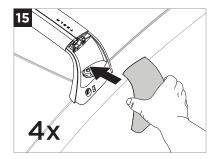
Install covers. Start with the bottom edge then press the top into place.
