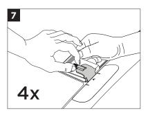
Keeping the clip tool in place, insert a clip (12) at the arrow location.
