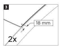
To locate the front arrows measure 18 mm from the front edge of the glass top.
