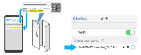
**NOTE:** If you are unable to connect to the Wall Connector SSID, turn off the cellular data function on your mobile device and try again.
