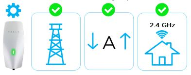
**NOTE:** To have the Wall Connector broadcast the SSID again, hold the button on the charge handle for 5 seconds or turn the circuit breaker off, then on again.
