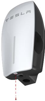
2. Use a T20 security pin Torx driver to remove the six screws on the sealing cover. Carefully remove the sealing cover and disconnect the ribbon cable. Save the screws and cover for reassembly.
