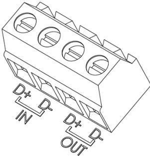
1. Form a daisy-chained network by connecting the cables from OUT to IN and
