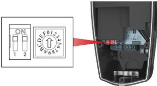
**⚠ Warning: Power MUST remain OFF** before setting or changing the DIP or rotary switches. Changing these switches with the power ON will not be recognized by the system and is dangerous due to the risk of electric shock.
