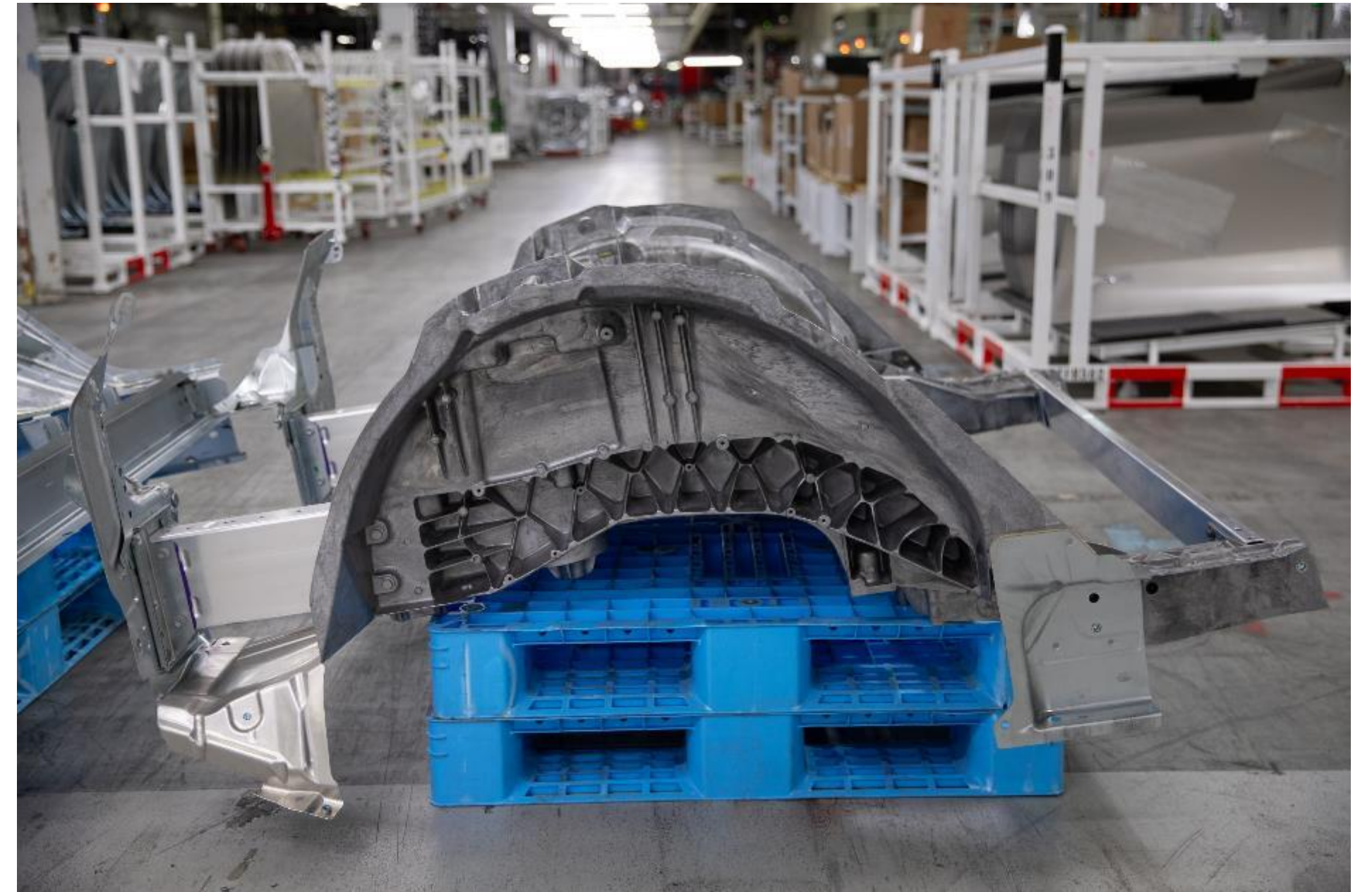
Model Y rear underbody 2 pieces of metal (eventually a single piece)
