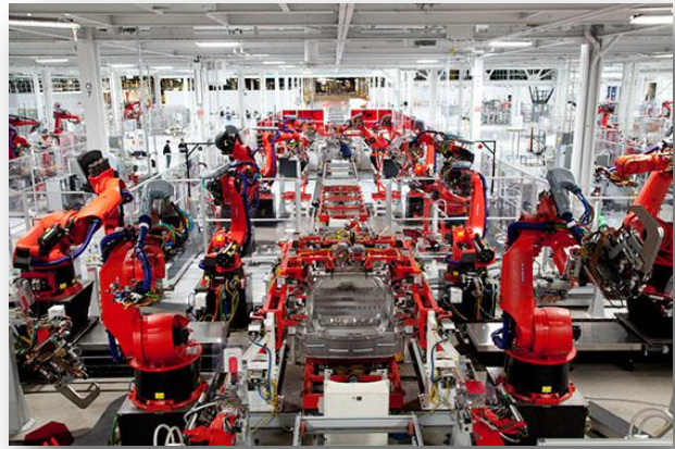
Body Assembly Robotics – Tesla Factory
