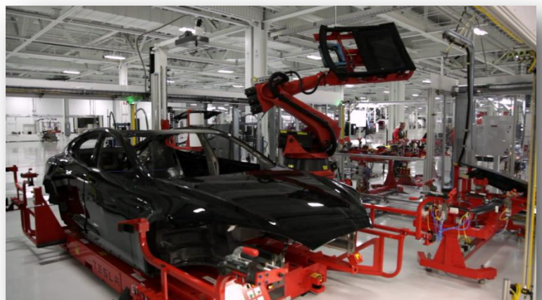
Robotic Installation of Panoramic Roof
