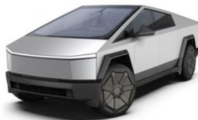
1. External body panels made of stainless steel.
